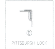
DUCT CONSTRUCTION DETAILS
